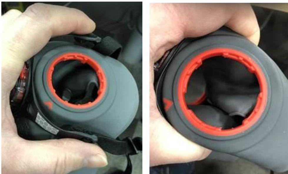
With your right hand, identify the White Arrow on the underside of the filter, just beneath the gasket. Your right hand being the dominant (stronger hand) will be used to orientate one of the filters.
